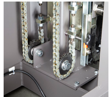
Flex S Series machines feature a dual chain film carriage lift for smooth and reliable fail-safe operation.
